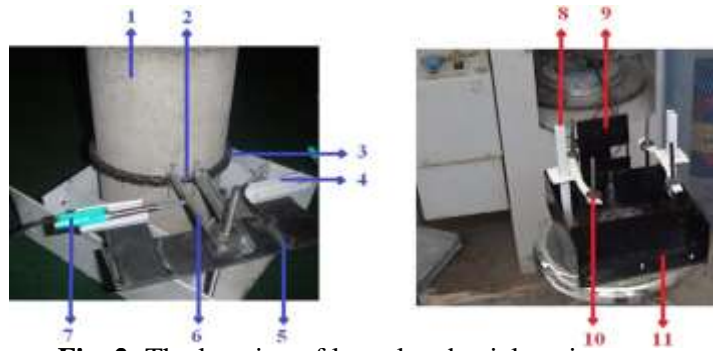
Fig. 2: The location of lateral and axial strain gauges.
